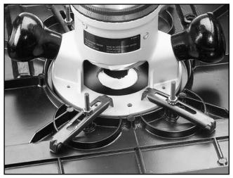
Figure 10. Correctly clamped router.
